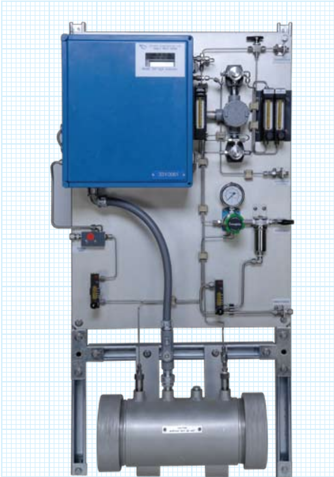
331 Total Sulfur complete with sample system
