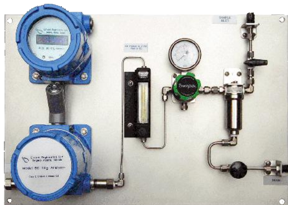
M60 with optional sample system mounted on 16" by 24" anodized aluminum panel
