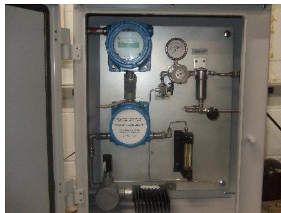
M60 with optional sample system in a heated fiberglass enclosure
